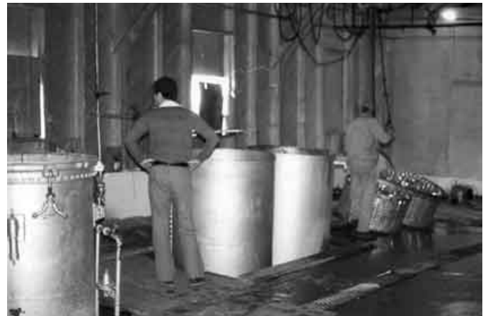
Figure 43. Steam kettles for sterilizing the canned oysters. The late Gilbert Maggioni is operating the overhead lift to remove the basket from the cooling vat. The sterilizing kettles are on the left behind W.D. Anderson (Keith photo, circa 1975).
