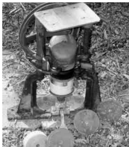
Figure 99. An electric can sealer (W. Collins collection).
