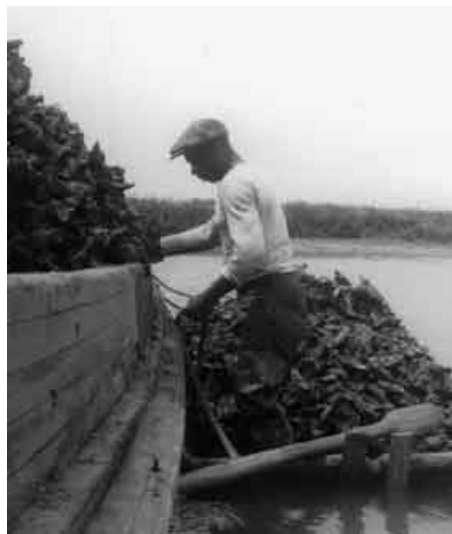
Figure 92. A wooden bateau with a load of oysters. Note the size of the handle on the oar and the sculling notch in the transom (Charleston Museum Photo, circa 1930s).
