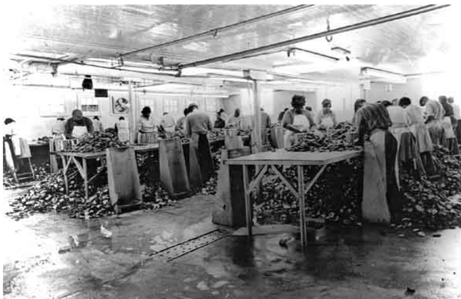
Figure 60. The shucking room at the Maggioni factory where oysters were opened for the raw shuck trade (Brown and Barton photo, circa 1950s).
