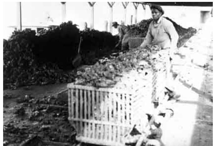
Figure 24. “Ten” bushel cars loaded with the oysters being pushed into the steam chests. Note that each was heaped up to increase capacity (Maggioni family photo).
