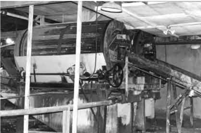
Figure 39. Shakers positioned over brine tanks so that as they rotated, oyster meats fell between gaps in metal rods into the tanks (Keith photo, circa 1975).
