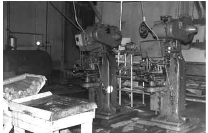
Figure 42. The filler and capper at the Maggioni Ladies Island facility (Keith photo, circa 1975).
