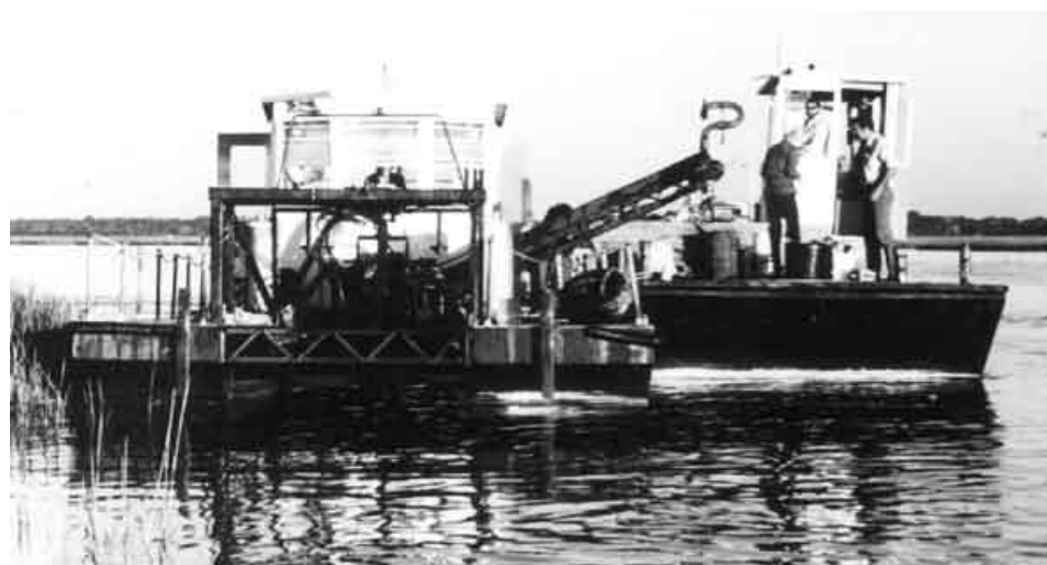
Figure 84. A mechanical harvester developed by Clemson University for use on intertidal beds (Keith photo).
