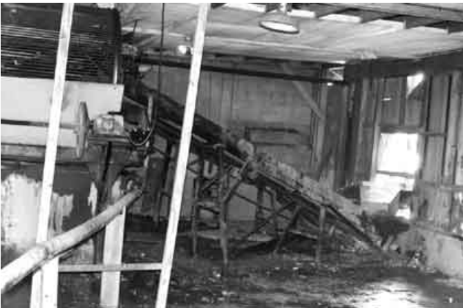
Figure 40. The chute from the shaker to the oyster pile for removal of shell from the shaker (Keith photo, circa 1975).
